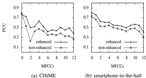
Figure 2: Pearson Correlation Coefficient (PCC) of 13 Low-Level Descriptors (i.e., MFCC 0-12) between the enhanced/non-enhanced speech and the clean speech over the whole test set with the *CHiME* noise (a) or the *smartphone-in-the-hall* noise (b).
